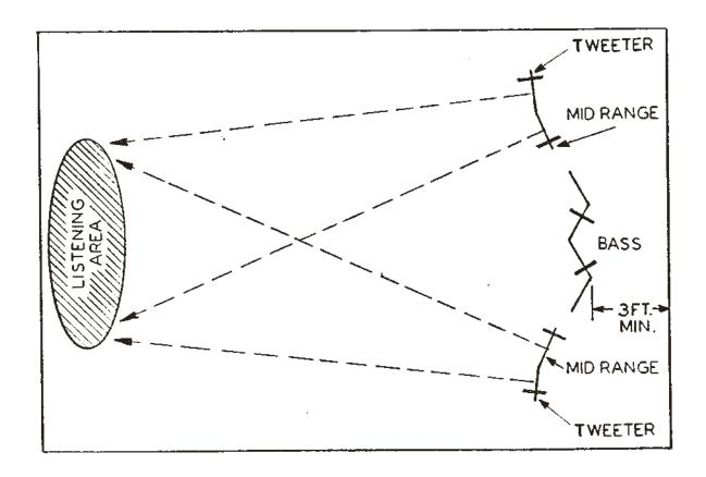
The speaker placement diagrams shown above are intended as a guide. As a general guide, these suggested installations will work in most listening rooms. The exact placement will vary for each room.
