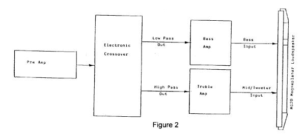
Set the high pass section at 200-300 Hz, 6dB per octave. Due to standing waves at the crossover frequency, the low pass section may require adjustment from as low as 90Hz (12dB Bessel) to 150Hz (15dB Butterworth). Typical settings are in the middle of this range. Optimization of the low pass can be done by ear (with music) or spectrum analysis.
